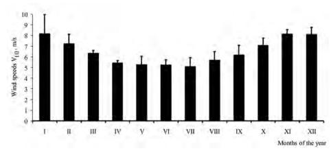
Fig. 3. Wind speeds in the work area at a height of 10 m above the water surface (according to data of the AHMS, located on the MLCPD-6).
