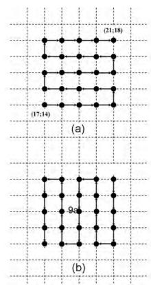
Fig. 5. Scheme of vessel «moving» within the calculation field in the dredging area: (a) – moving from the node with grid coordinates (17; 14) to the node with grid coordinates (21; 18); (b) is a reverse movement from a node with grid coordinates (21; 18) to a node with grid coordinates (17; 14).
