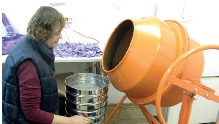
Photo 4 – Working with the “Ballerina” (a name lovingly given to a concrete mixer) – simulating the periodic mechanical action of bottom sediment on the fragmentation of plastic fragments in the wave-surf zone. Filtration procedure. Kaliningrad, 2015. (photo – E. Esiukova)
