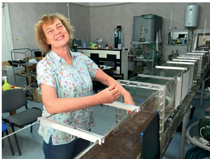
Photo 3 – During preparation for an experiment on the movement of microplastic particles of different shapes. Hydroflume at the Atlantic Branch of the Shirshov Institute of Oceanology, Russian Academy of Sciences, 2019. (photo – E. Esiukova)
